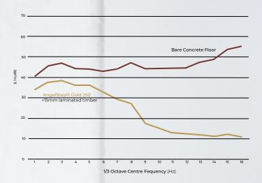
In the case above, AngelStep® 250 in a 3 layers system, installed under a 15mm laminated timber, was one of the best performing system in terms of floor impact noise improvement compared to the base floor, with improvement of up to 31 points in the L'nT,w rating; a result similar to a high pile carpet installed over a high quality underfelt.
